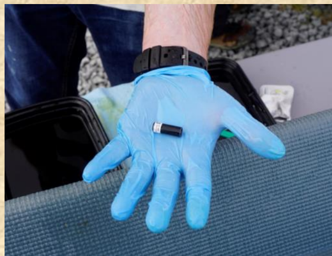
Figure 4: An Innovasea V9P-2x-180kHz HR acoustic tag with depth sensing capability up to 30 m. Tags transmit a signal every ~3 seconds (John Sanna 2022).
