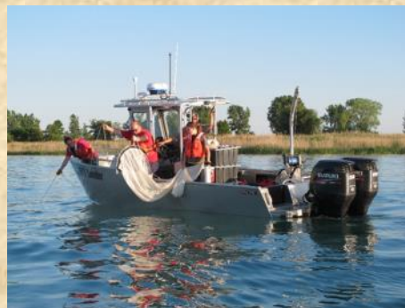
Setting a D-frame net to collect drifting larvae in the St. Clair River. Credit: USGS GLSC.
