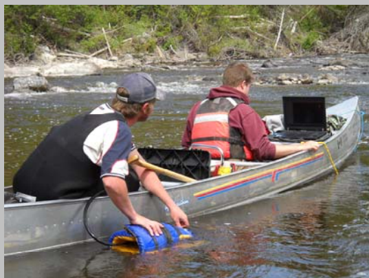
Photo left: A Trent University grad student and a DFO intern survey the spawning substrate using a DIDSON sonar.
